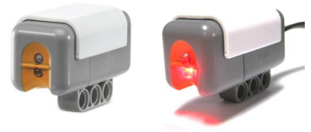
Figure 1.7 – Light Sensor in ambient mode (left) and reflected mode (right)
